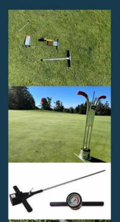
Probe/Lateral Profile - Allows turf managers to visualize and measure essential metrics such as thatch, root depth, and layering in the soil profile.
